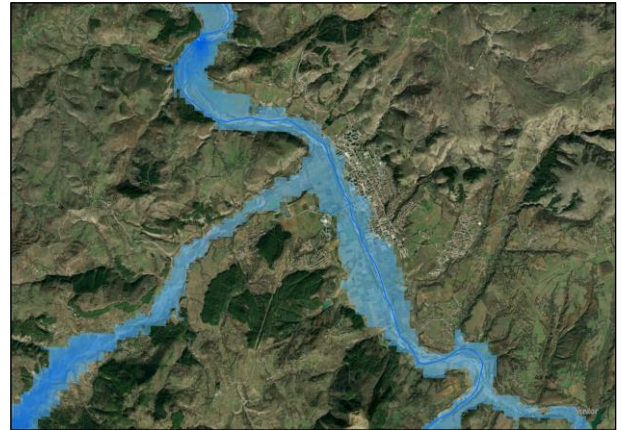
Figure 2. Modelled depth of the water layer.
